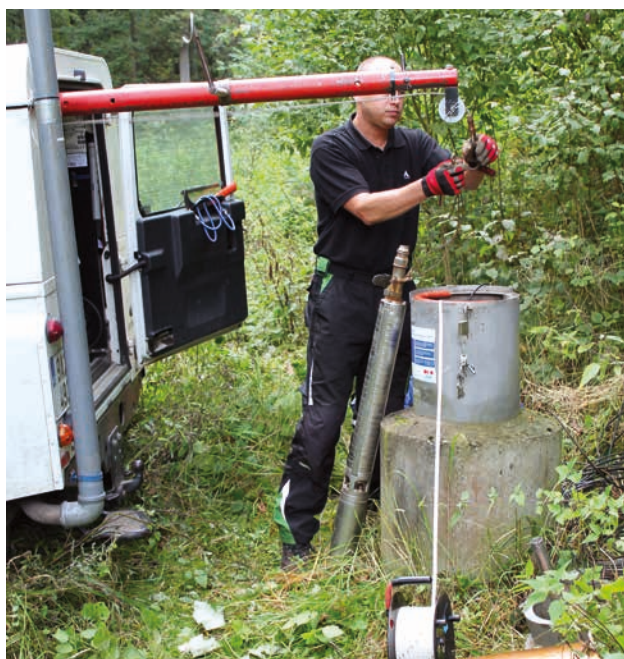
Inserting the pump into the borehole before sampling the groundwater (source: Czech Hydrometeorological Institute)
