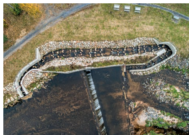
Fish crossing, the Smědá Stream in Frýdlant (source: Elbe River Board, s.e.)
